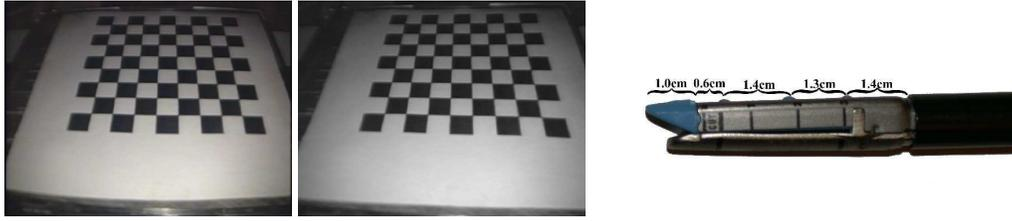
Figure 1: (left) Original image obtained from a  $35^\circ$  endoscope. (center) Image after undistortion. (right) Stapler instrument with identifiable points and known measurements.
